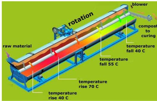
**Figure 4. Rotary drum**
