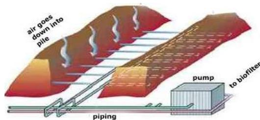
**Figure 3. The aerated static pile**
