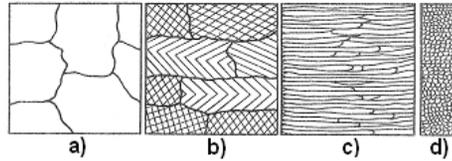
Figure 1 – Changing of crystal grain size in structure after cold deformation of sheet:
