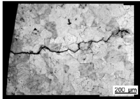
**Figure 4 – One intercrystal crack in 585 gold jewel alloy**
