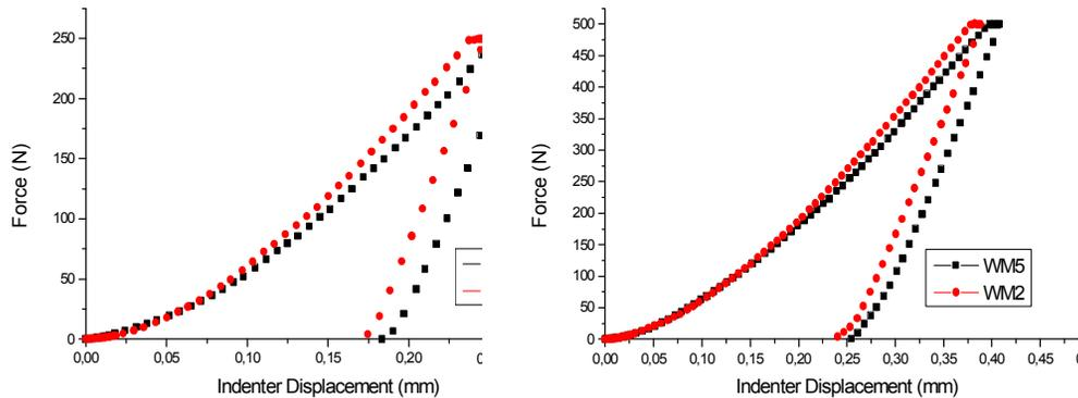
**Figure 3. Force-indentation displacement curves showing the loading and unloading curves for two different tin-based bearing materials under 250 and 500 N force**
