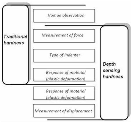
**Figure 1. Schematic presentation of the measurement parameters of traditional and depth sensing hardness test methods**
