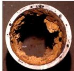
**Figure 3 – Pit cast pipe showing porosity (black dots on cut metal surface) [5].**
