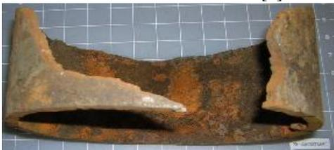
**Figure 1 – Heavily corroded gray cast iron pipe**
