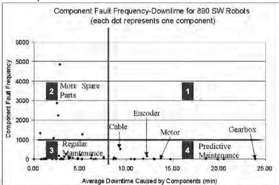
Figure 2 - Four quadrant chart for identifying critical components
