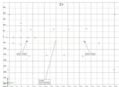
**Figure 4.** Measure of 500mm gauge block in measuring project with factory-equipped coded reference points
