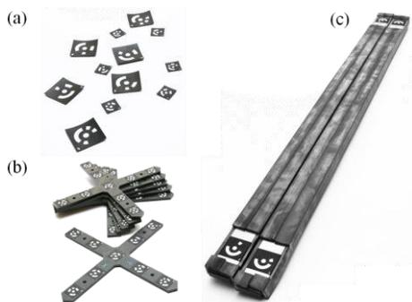
**Figure 1.** Reference objects of photogrammetric system: (a) coded reference points, (b) orientation crosses, and (c) reference scale bars
