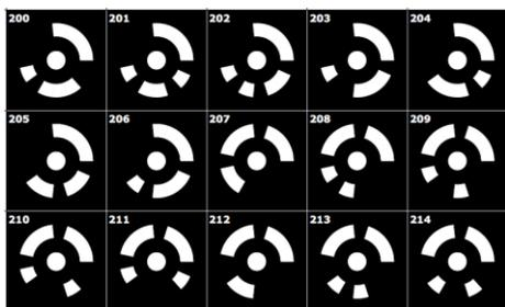
**Figure 2.** Sheet of paper sample with user-generated coded reference points
