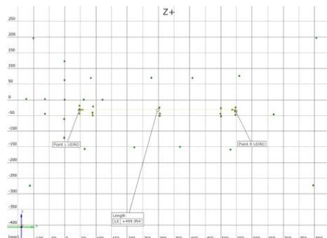
**Figure 5.** Measure of 500mm gauge block in measuring project with user-generated coded reference points
