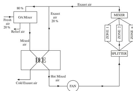
**Figure 1** - Simplified mechanical ventilation system with HR unit
