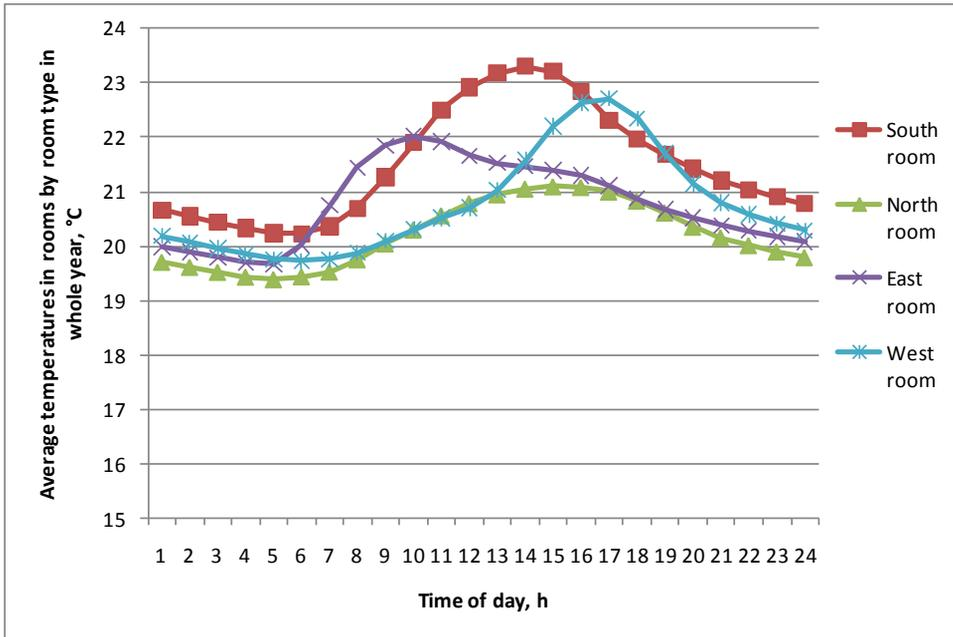
**Figure 4.** Average temperature in rooms during whole year when FullInteriorExterior solar radiation model is used
