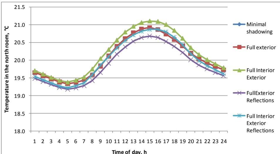
**Figure 5.** Average temperature in the north room during a year by different solar radiation model
