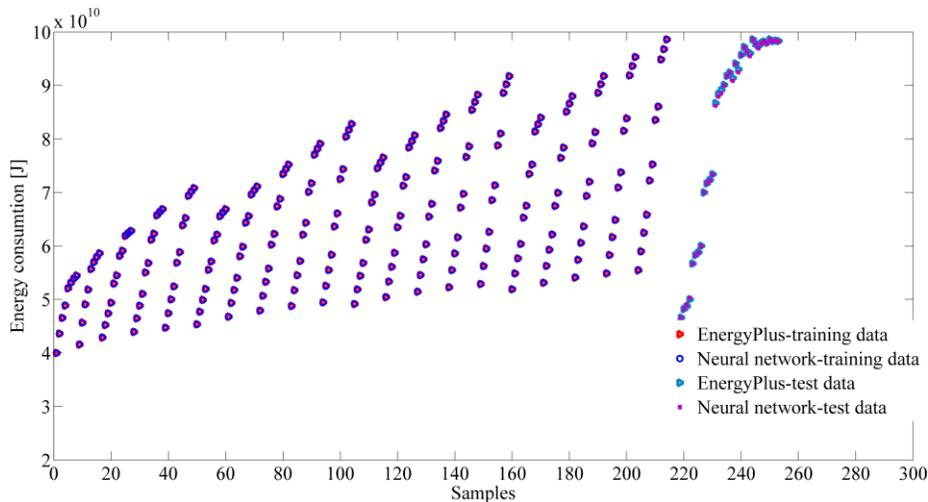
**Fig. 2.** EnergyPlus simulated and MLP model computed values of energy consumption in training and test sets.
