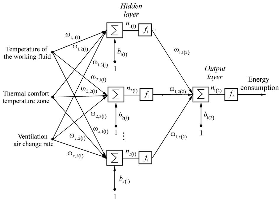
Fig.1. The two-layer perceptron neural network.
