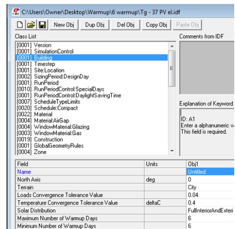
**Figure 2. Input dialog for maximum and minimum number of warm-up days**
