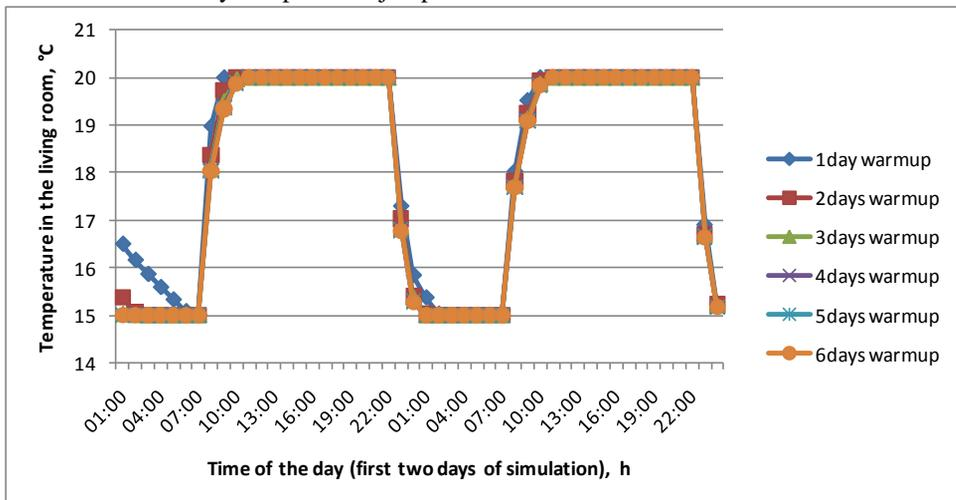
Figure 5. Temperature in the living room during first two days of simulation when thermostatic valves are installed
