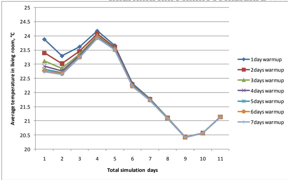
Figure 4. Average temperatures in first 11 days of simulation depending on number of warmup days
