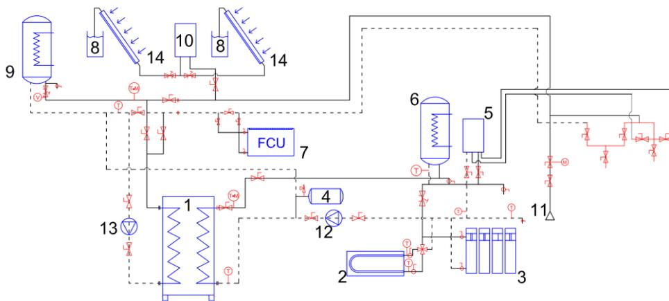
Figure 4. Hydraulic schema of existing installation of heat pump and solar collectors
