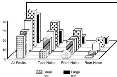
**Figure 2. Market research data showing severity of brake noise problem (failures per 100 vehicles) [5]**
