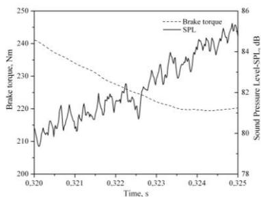
**Figure 6. Influence of the brake noise's appearance on the brake efficiency for maximum pressure of 2.5 MPa and an initial speed of 714 rpm ( $v=70$  km/h)**
