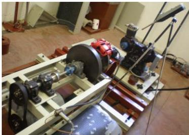
**Figure 4. Photo of laboratory installations designed for the brake noise investigation**
