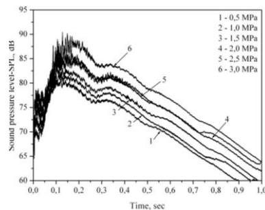
**Figure 8. Variations of the sound pressure levels for the initial disc speed of 765 rpm ( $v=75$  km/h)[9]**
