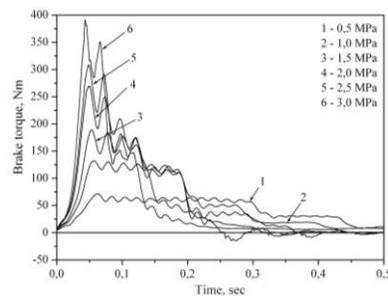
**Figure 7. Variation of the braking torque for the initial disc speed of 765 rpm ( $v=75$  km/h[9])**
