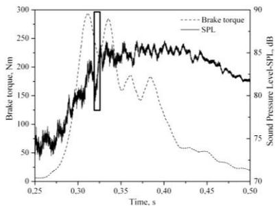
**Figure 5. The braking torque and SPL-maximum pressure of 2.5 MPa and an initial speed of 714 rpm ( $v=70$  km/h)[9]**
