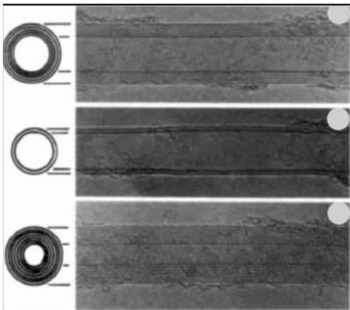
**Figure 1. Transmission electron micrographs (TEMs) of the first observed multi-wall carbon nanotubes reported by Iijima in 1991 [4]**
