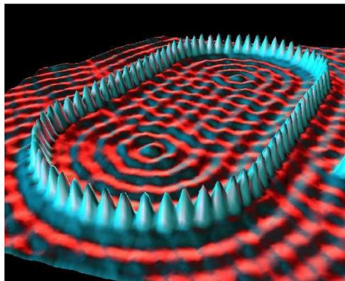
*Figure 2. Scanning Tunneling Microscope (STM) image of density of electron states for a corral of Fe atoms on a Cu metal surface [13]*
