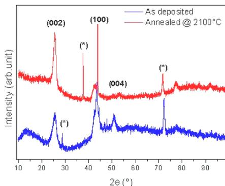
**Figure 3. XRD spectra of CNT where (\*) is the difference peak of CNT [14]**
