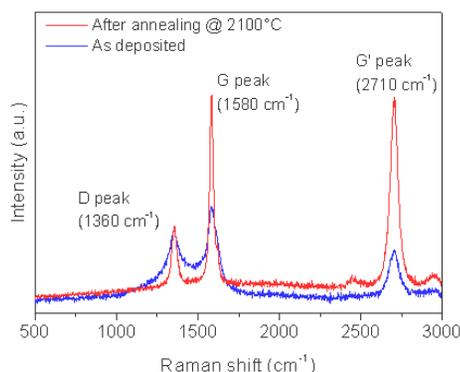
**Figure 4. Raman spectra of CNTs [16]**
