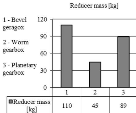
Figure 7. Comparison of drives according to mass
