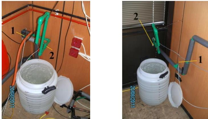
**Figure 6. View of the volumetric tanks and positions of the electric thermometers for the BFPC (left) and the FPC (right): 1 - Pt-100 resistance thermometer at the inlet of the solar collector and 2 - Pt-100 resistance thermometer at the outlet of the solar collector**
