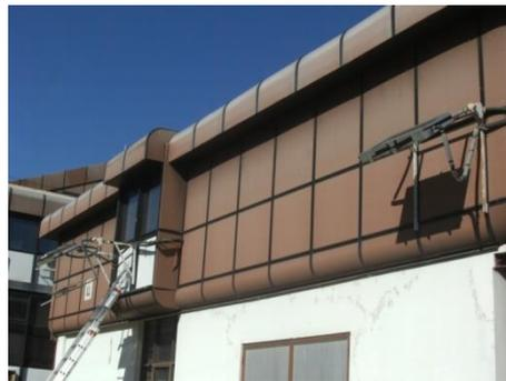
**Figure 4. The FPC (left) and the both analyzed collectors (right)**
