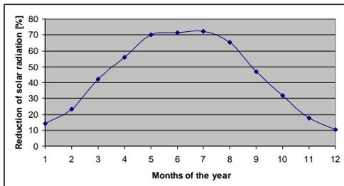
**Figure 2. The percentage reduction of solar radiation that passes through the windows due to the influence of horizontal roof overhangs**
