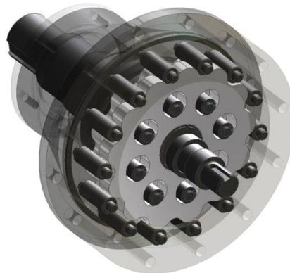
**Figure 1. Model of cycloid drive**
