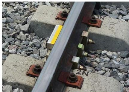
**Figure 7. Wheel Condition Monitor (WCM) [28]**
