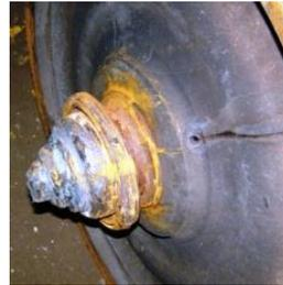
*Figure 5. Broken wrist axle assembly*
