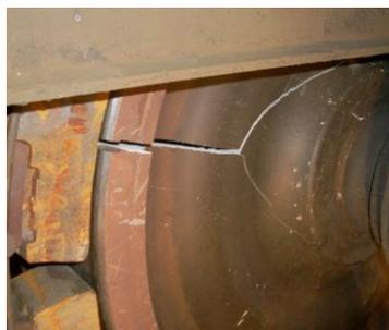
**Figure 2. Rupture of wheel**
