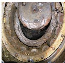
*Figure 4. Heated axial bearing*
