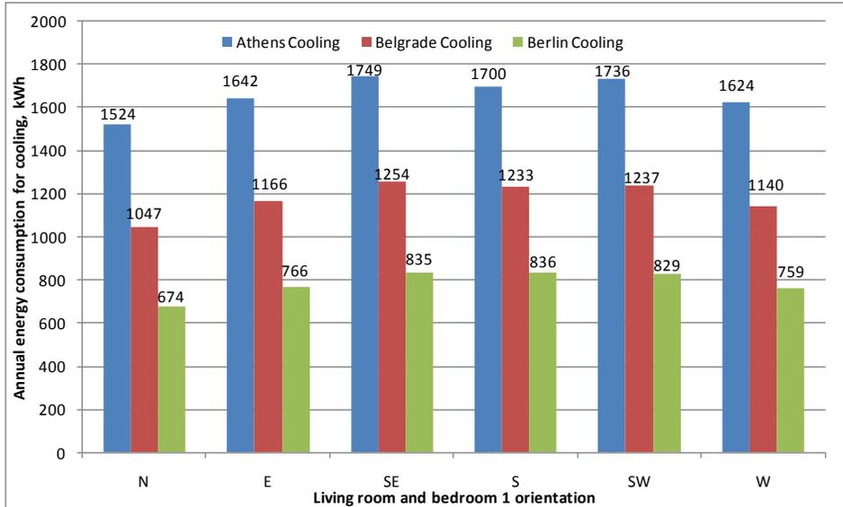
Figure 4. Energy consumption for cooling depending on the orientation and location
