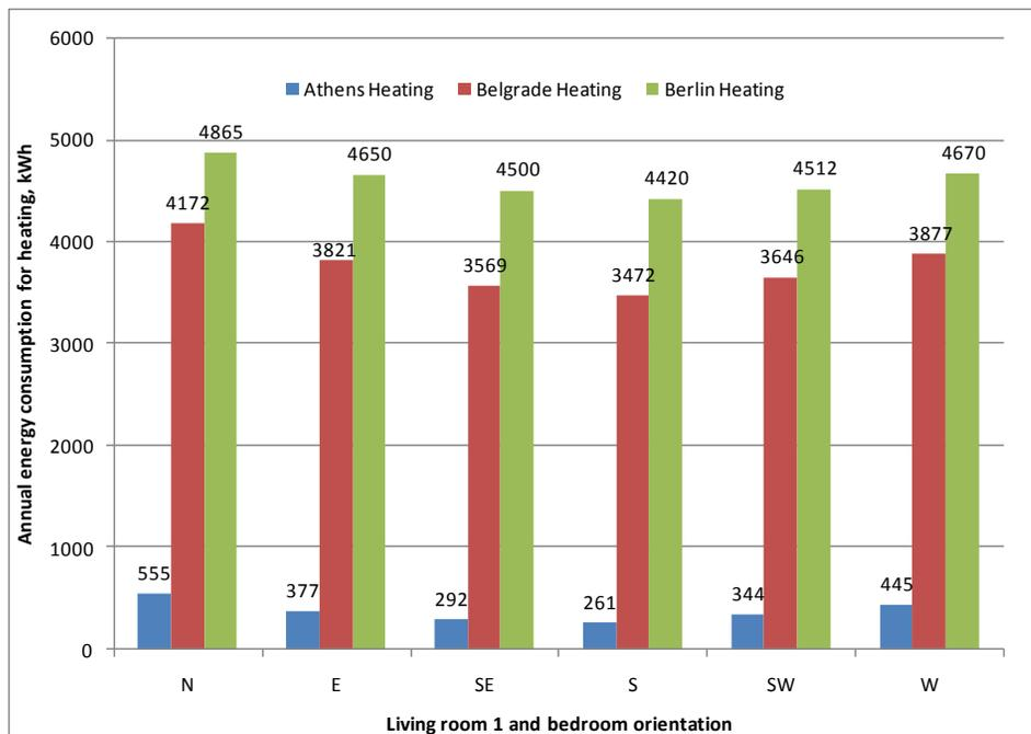
**Figure 3. Energy consumption for heating depending on the orientation and location**
