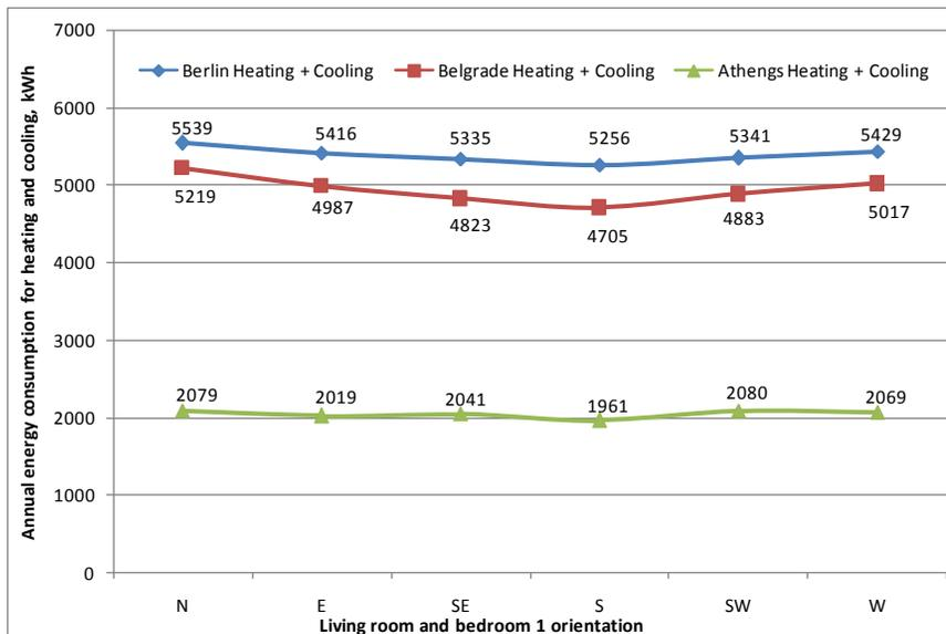
Figure 5. Energy consumption for heating and cooling depending on the orientation and
