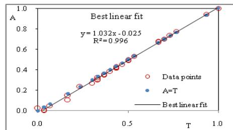
**Figure 10.  $R^2$  value between estimated and measured data in learning process for  $L_{eq}$  (1h)**
