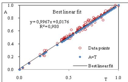
**Figure 6.  $R^2$  value between estimated and measured data in learning process for  $L_{eq}$  (15 min)**
