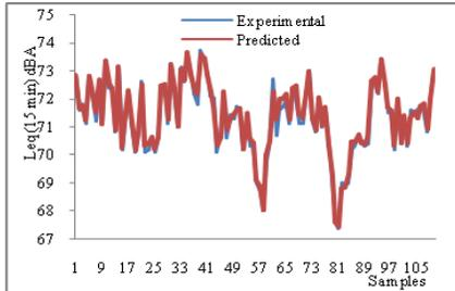
**Figure 5. The difference between predicted and measured values in learning process for  $L_{eq}$  (15 min)**
