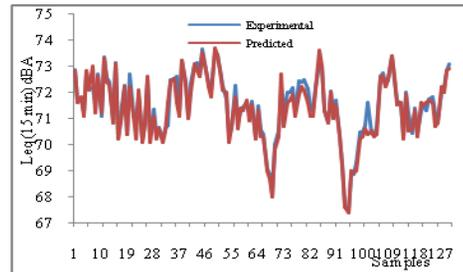
**Figure 7. The difference between predicted and measured values for whole data set for  $L_{eq}$  (15 min)**
