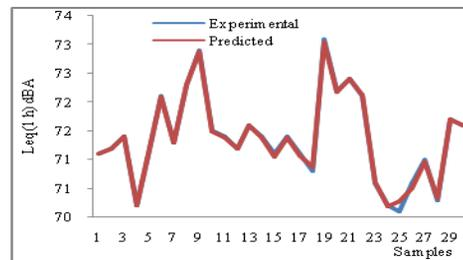
**Figure 9. The difference between predicted and measured values in learning process for  $L_{eq}$  (1h)**
