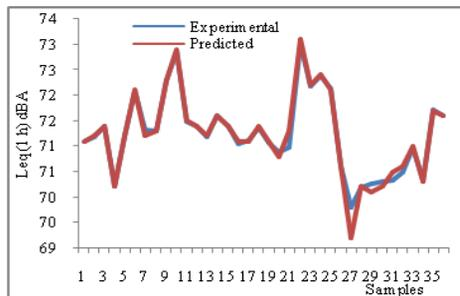
**Figure 11.** The difference between predicted and measured values for whole data set for  $L_{eq}(1h)$
