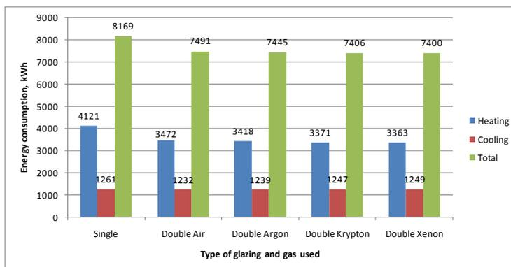
**Figure 5. Energy consumption when single and double glazing is used by gas type selection**
