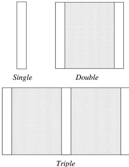
**Figure 3. Type of glazing (intersection view, clear block presents glazing, dotted block presents gas)**
