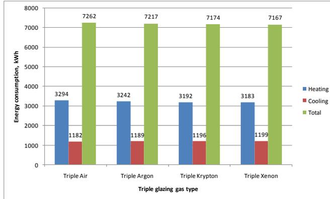
Figure 6. Energy consumption when triple glazing is used by gas type selection
