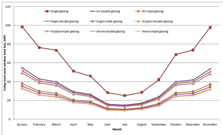
Figure 8. Living room zone window heat loss energy
